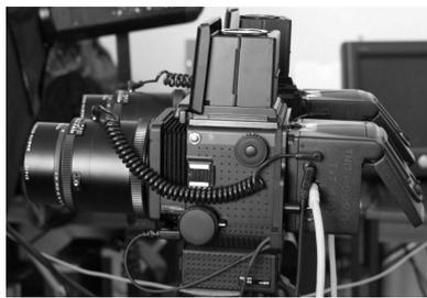
*Figure 3: Colour camera used in the stereo pair*
